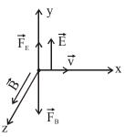
Directions of electric force (  $\vec{F}_{_{E}}$  ) & magnetic force (  $\vec{F}_{_{B}}$  ) are just opposite.
