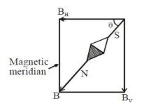
$B \Rightarrow$  resultant magnetic field of earth's magnetism  $B_H \Rightarrow$  Horizontal component  $B_V \Rightarrow$  Vertical component
