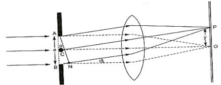
Path difference between the secondary waves reaches at point P
